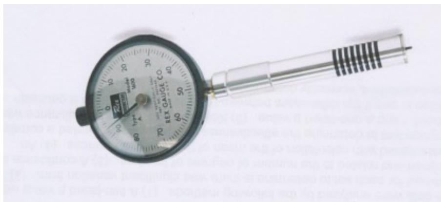
**Fig. 1.** Rex Gauge durometer®. The pressure sensitive pin is seen at the base of the instrument. The instrument has a manual calibration and reset button at the top of the dial with measurements from 0 to 100.
