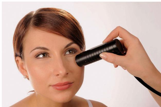
**Fig. 2.** Courage-Khazaka cutometer® MPA 580 — with the handpieces stored on top. Measurements are taken using the cylindrical handpiece applied to the skin. The handpiece has a suction port at the tip into which the skin is withdrawn and released. The device is connected to a PC with data entered automatically into a program to analyze the curves produced.
